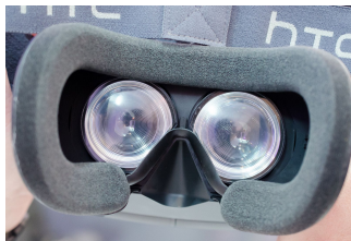
Figure 1. Lenses in HTC Vive
